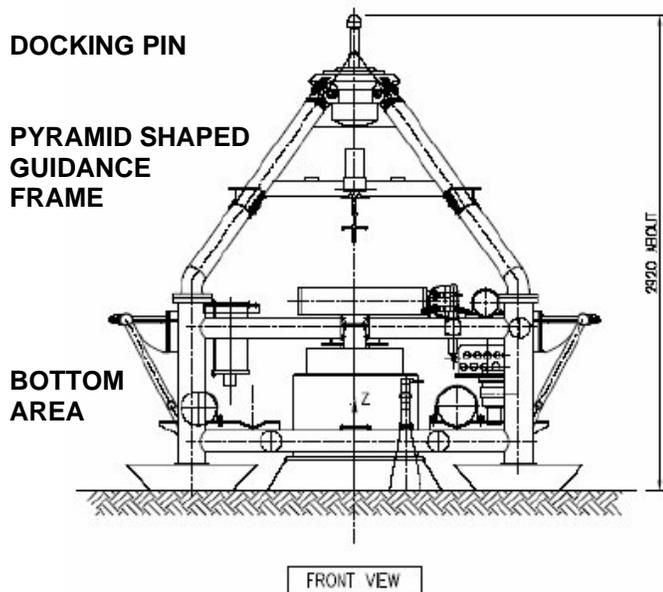
Fig. 2 Bottom Station of MABEL with equipment and docking pin on top – the footprint of the base is 3000 mm x 3000 mm.
