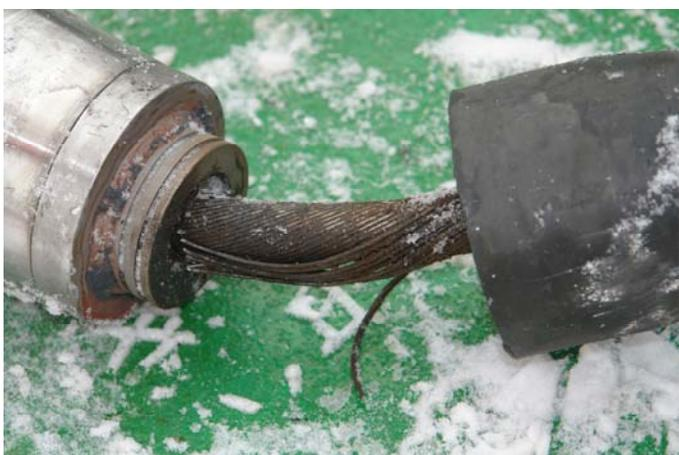
Fig. 13 Detail of the umbilical termination after operation. Left: pressure housing connected to the top of MODUS. Right: bending restrictor completely pushed aside due to strong roll and pitch. Mid: umbilical with broken wires of the outer armouring layer.
