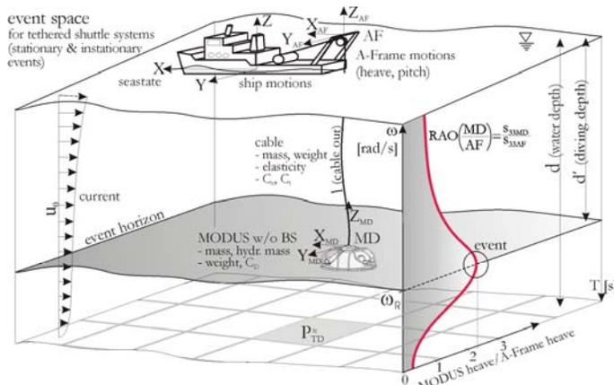
Fig. 6 Event space for tethered shuttle systems: stationary and instationary events. Influences on dynamic behavior of MODUS during sea operation – general terms.
