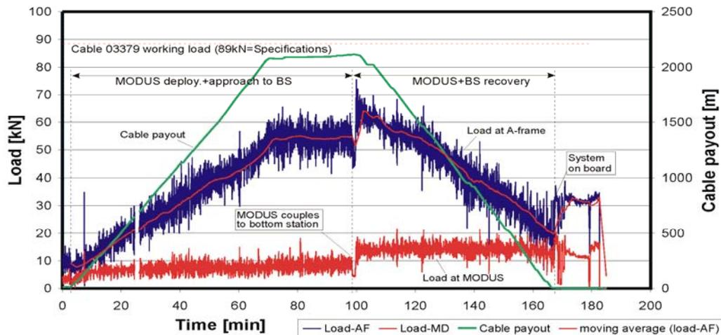
Fig. 8: Profile of load at A-frame (AF) and at MODUS (MD) with cable payout during a complete operations cycle for recovery of a bottom station from 2000 m; ( $m_0$  MD=1090 kg,  $m_0$ -BS=1433 kg)
