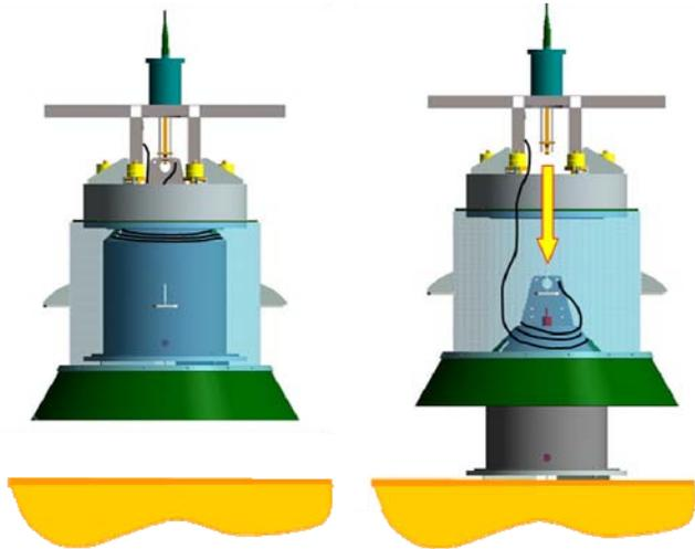
Fig. 4: Cross cut view of the design study of the Seismometer, with the outer shell during deployment (left) and the sea floor operation (right).
