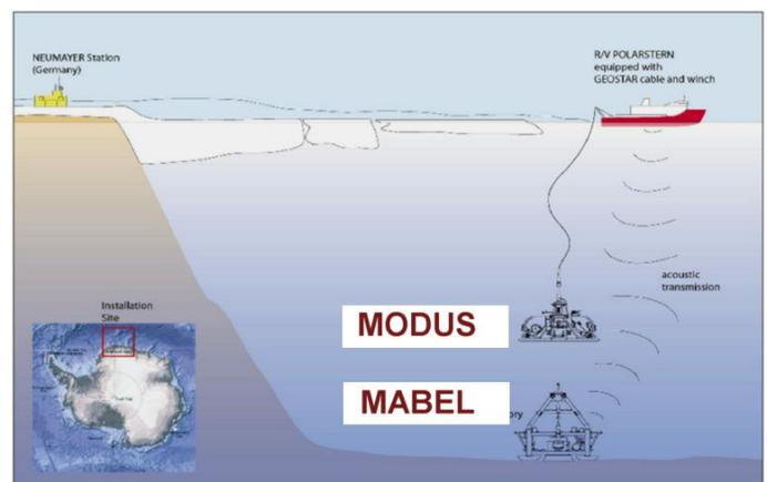
Fig. 1: Scenario of the recovery procedure of the MABEL station. R/V Polarstern as carrier of the docking module MODUS close to the shelf ice edge. Operational depth 1850 m.
