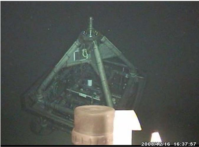
Fig. 19 MODUS approaching MABEL at a water depth of 1837 m shortly before docking.
