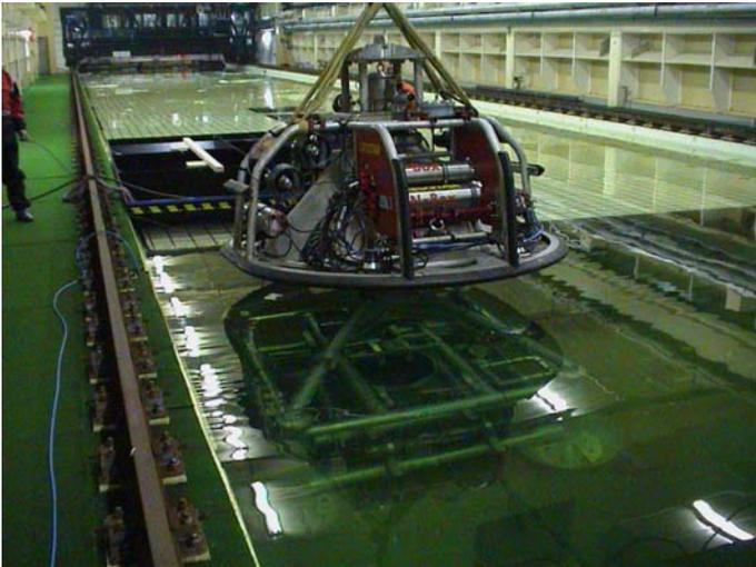
Fig. 9: MODUS and MABEL during the environmental tests in the large ice tank of the HSVA in 2002.
