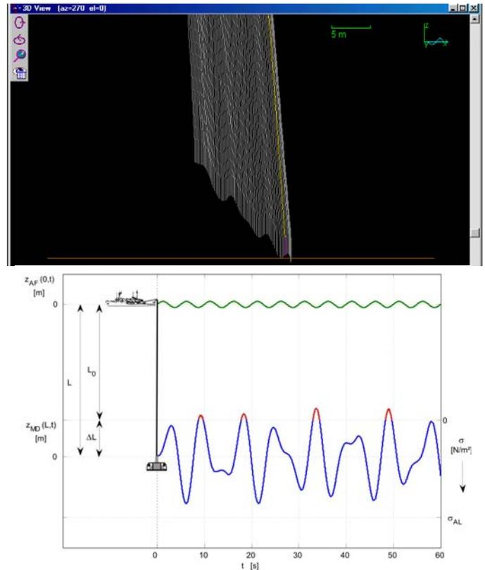
Fig. 7 top: Simulation model of RV and MODUS. Operation close to sea bottom – time line. Results: Orcaflex simulation run by Tecnomare S.p.A. bottom: Principle of MODUS motion in the event space by wave motion induced from the research vessel (meter of motion vs. time – relative data, non-scaled).
