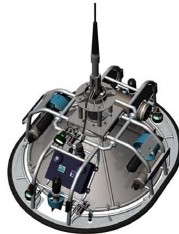
Fig. 5: Design study of MODUS showing the umbilical connection on top, the transformer at the front, the thruster for positioning, the cameras, and the lighting arrangement. Weight in air 10 kN, in water 7 kN; H 1700 mm, W 2300, L 3200 mm.
