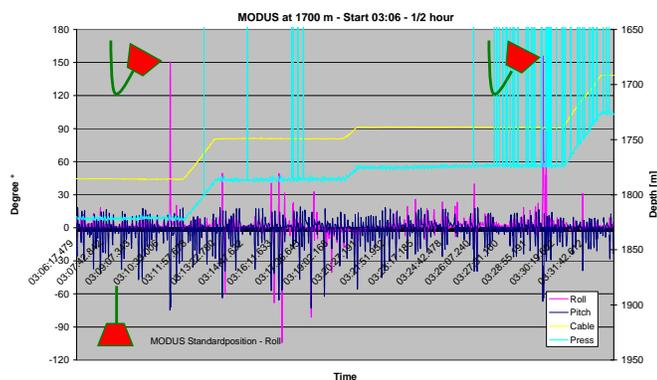
Fig. 12 Last hour of the search operation. Clear indication of extreme events: roll (magenta) and pitch (blue)  $> 90^\circ$ . Pitch can be compensated by the flexible bearing of the termination, roll cannot. Operational depth is indicated by cable payout (yellow) and related pressure (cyan). Spikes in pressure indicate transmission failure of the fibre optic line.
