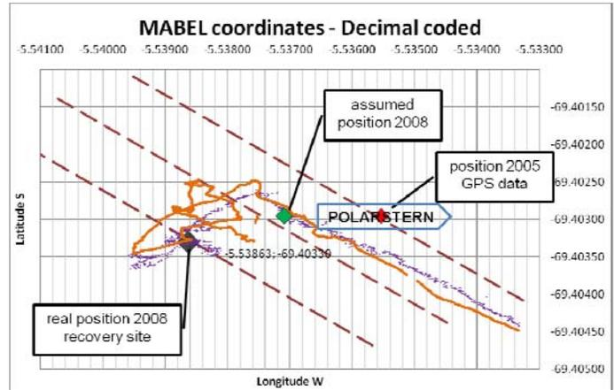
Fig.21 Search tracks December 16<sup>th</sup>, 2008: Polarstern (orange). MODUS with Posidonia (purple). Red spot: deployment position: Lat 69° 24,295'S Lon 5° 32,220'W. Assumed position of the station (green), real position on the sea floor (deep purple – large spot on the lower track).
