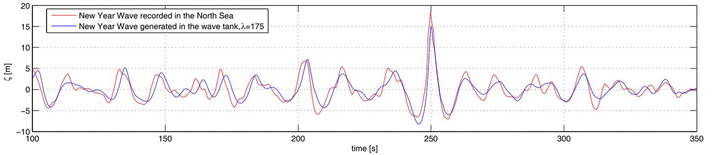
Figure 4. OPTIMIZED WAVE TRAIN AT TARGET POSITION ( $x = 6$  m, WATER DEPTH  $d = 0.4$  m, 70 m FULL SCALE) AFTER 23 ITERATION STEPS IN COMPARISON WITH THE RECORDED NEW YEAR WAVE SEQUENCE (WAVE TANK SIMULATION AT SCALE 1:175, PRESENTED AS FULL SCALE DATA).
