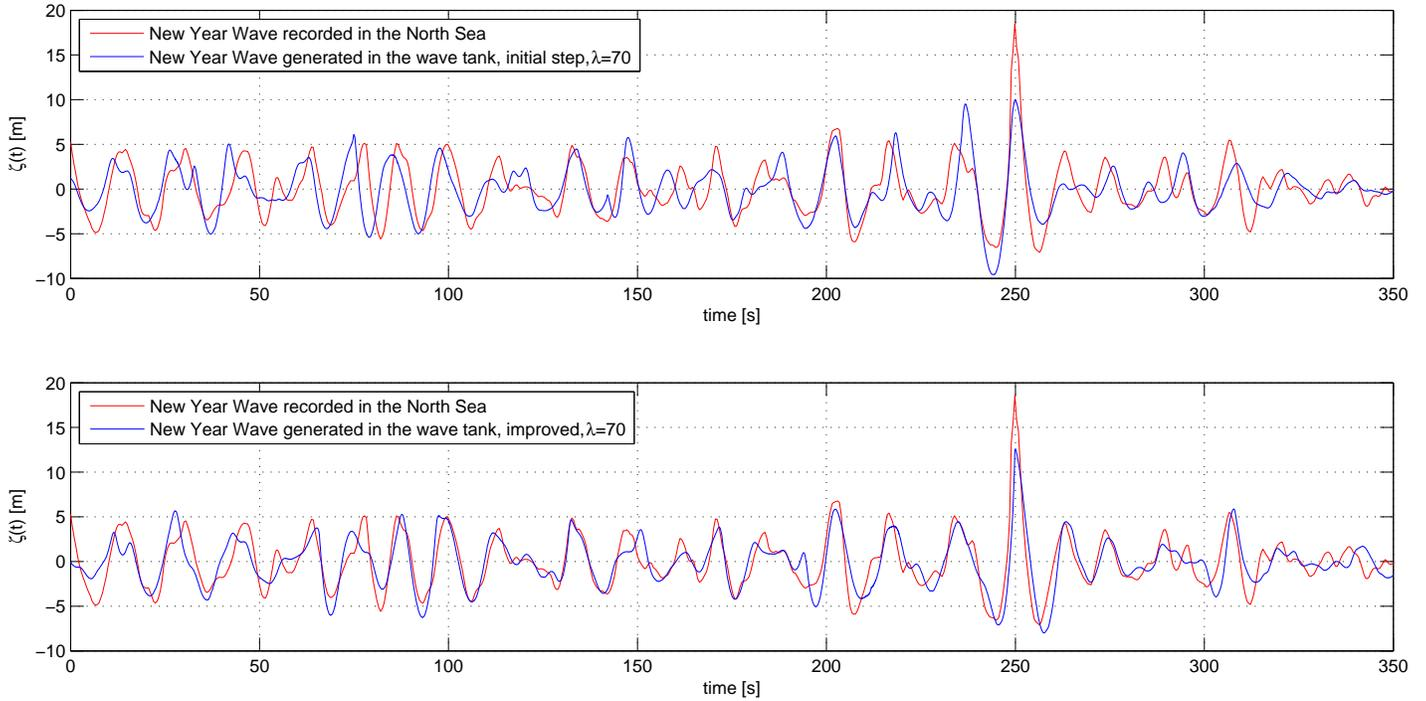
Figure 2. OPTIMIZED WAVE TRAIN AT TARGET POSITION ( $x = 50$  m, WATER DEPTH  $d = 1.0$  m, 70 m FULL SCALE) AFTER ONE ITERATION STEP OF THE PHASE-AMPLITUDE ITERATION SCHEME IN COMPARISON WITH THE RECORDED NEW YEAR WAVE SEQUENCE (WAVE TANK SIMULATION AT SCALE 1:70, PRESENTED AS FULL SCALE DATA).
