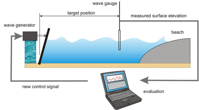
Figure 1. OPTIMIZATION OF MODEL WAVES. THE WAVE SEQUENCE IS GENERATED, MEASURED, EVALUATED AND MODIFIED IN ORDER TO IMPROVE THE WAVE QUALITY WITH RESPECT TO THE TARGET WAVE TRAIN.
