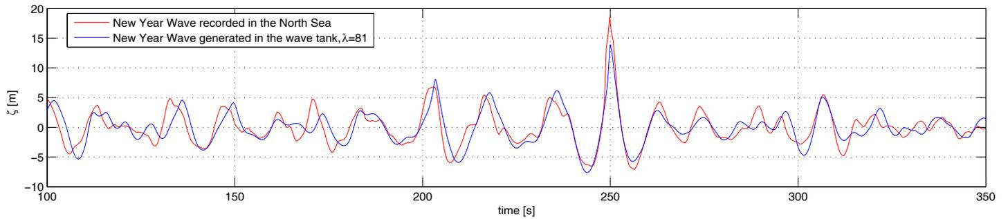
Figure 3. OPTIMIZED WAVE TRAIN AT TARGET POSITION ( $x = 30$  m, WATER DEPTH  $d = 1.5$  m, 121.5 m FULL SCALE) AFTER TWO ITERATION STEPS OF THE PHASE-AMPLITUDE ITERATION SCHEME IN COMPARISON TO RECORDED NEW YEAR WAVE SEQUENCE (WAVE TANK SIMULATION AT SCALE 1:81, PRESENTED AS FULL SCALE DATA).
