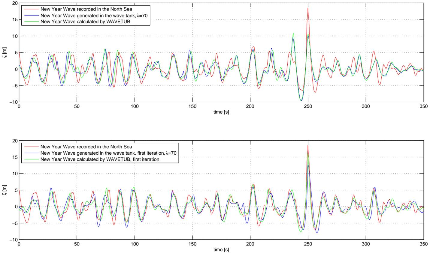
Figure 7. TOP: NUMERICAL SIMULATION AND WAVE TANK REALIZATION RESULTING FROM THE SAME INITIAL CONTROL SIGNAL; BOTTOM: NUMERICAL SIMULATION AND WAVE TANK REALIZATION BASED ON (DIFFERENT) IMPROVED CONTROL SIGNALS APPLYING THE PHASE-AMPLITUDE ITERATION SCHEME.
