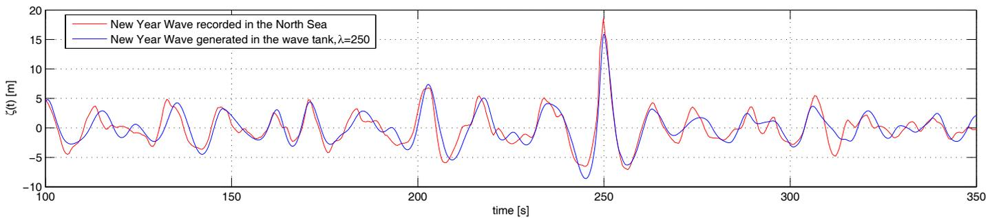
Figure 5. OPTIMIZED WAVE TRAIN AT TARGET POSITION ( $x = 6$  m, WATER DEPTH  $d = 0.4$  m, 100 m FULL SCALE) AFTER TEN ITERATION STEPS IN COMPARISON WITH THE RECORDED NEW YEAR WAVE SEQUENCE (WAVE TANK SIMULATION AT SCALE 1:250, PRESENTED AS FULL SCALE DATA).
