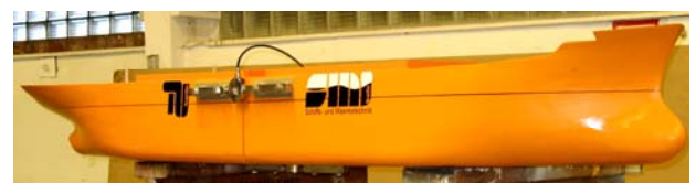
Fig. 3: Model of the segmented bulk carrier at model scale 1:70
